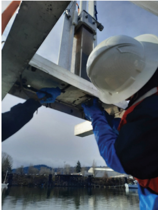
Photo 1 Inserting SedFlume piston seal
