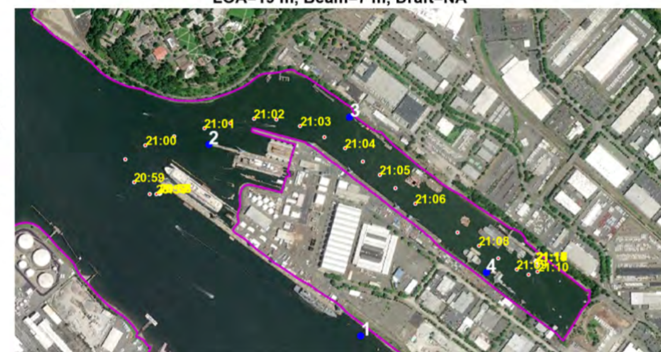
Figure 3-16 Vessel Wake Event Identified in Swan Island Basin at Station 3
