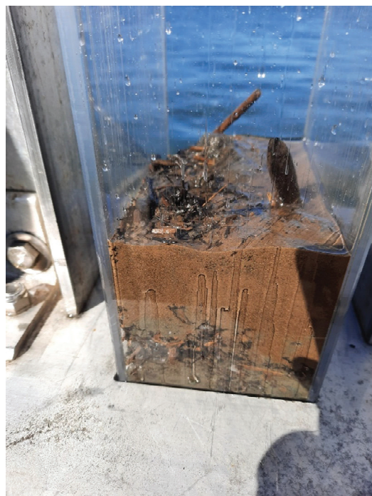
Photo 2 Example low recovery SedFlume core due to wood debris
