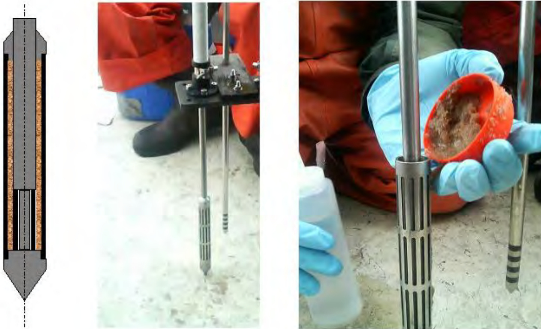
Figure 5. Trident porewater sampler with sand-pack system.
